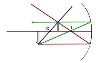
7. Construct the image on the drawing below via ray tracing.
