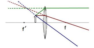
10. Construct the image formed by the object as shown below. If the focal length of the lens is 15.5 cm and the 3.20 cm (in height) object is placed 22.0 cm from the lens, find (a) the image distance, (b) the magnification, (c) the image height.
